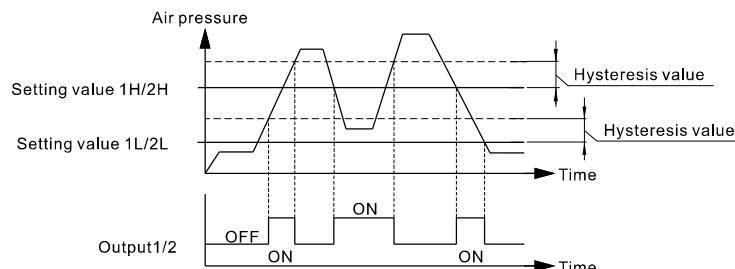
4. Suction check mode: Generally used for suction check detection applications. After the zero-shift signal is triggered, the zero-shift is completed after the TS time.
